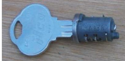
Ilco 1573A inserted in cylinder plug
