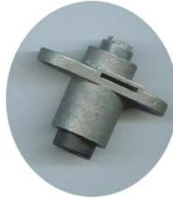
In they above picture you see lock body with plug and driver. You also see a slot where you can insert a broken pick or very small screwdrivers and push down the retainer wafer to remove the plug out of the lock body.
