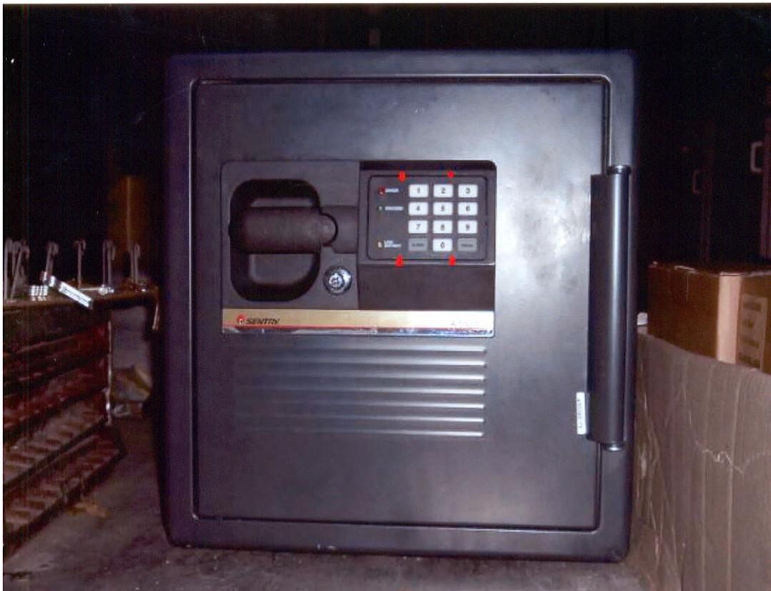
On the front of the safe in this picture there are four red dots. These dots mark the location of the tabs holding the keypad on the safe. Gently insert a thin blade screw driver at these points pushing in and down gently to remove the cover. The rubber keypad will come out with it. With the cover removed the circuit board is exposed.
