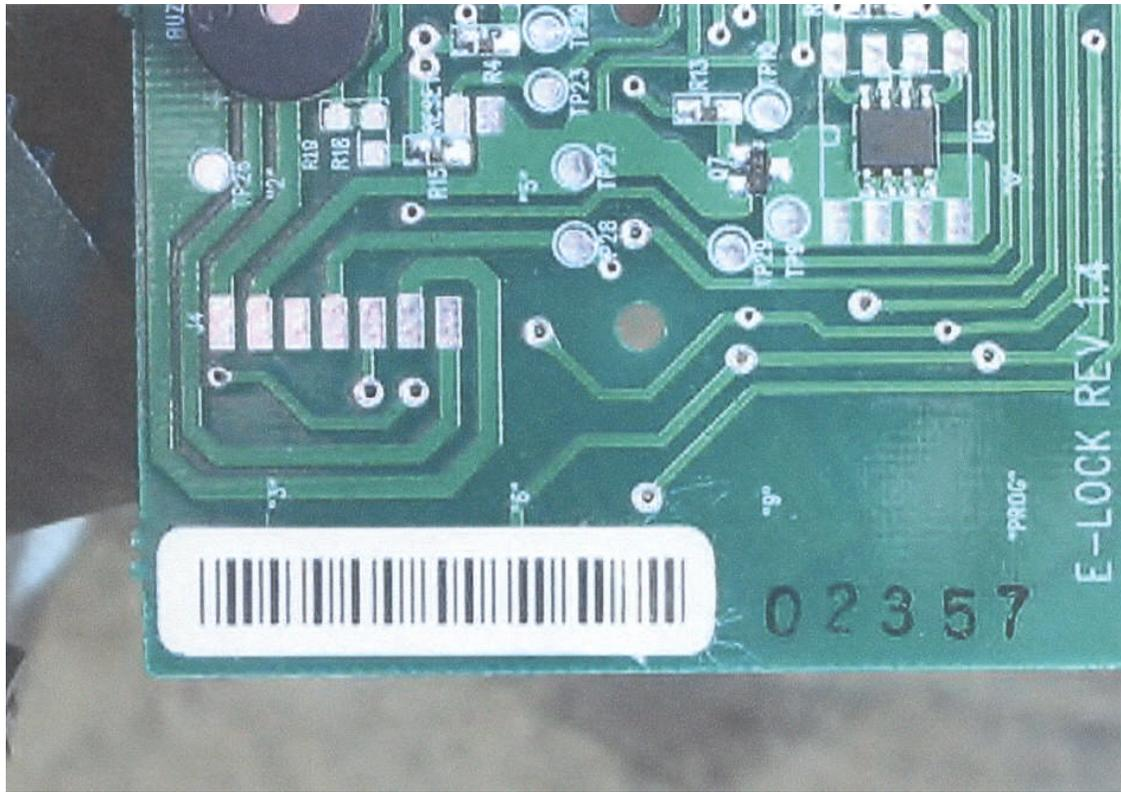
There are seven groups of bars in the barcode on the circuit board. You ignore the first group and the last group of bars. Within the remaining 5 groups there are generally 5 bars per group. The first three bars in each of these groups are what will be used to decode the combination.
