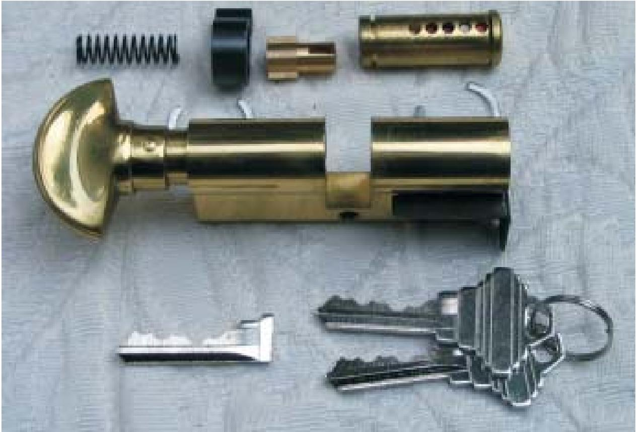
Start by placing this cylinder with the bible in the vise. Using two small flat screwdrivers, one to hold one of the retainer C clip's end in place the other to bend the same retainer C clip away from the cylinder body. Do the same with the second retainer C clip, the C clips are made from a soft material and will be reused after rekeying the cylinder.
