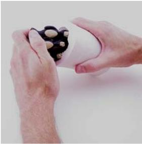
6. Once the mold has been removed from the mold box, flex the cured silicone mold and remove your original. You now have a perfect mold of your unharmed original. You are now ready to make identical castings of your original.
