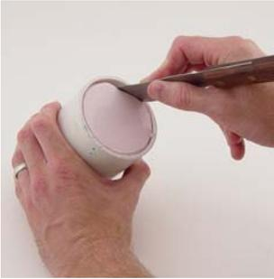
5. Let the rubber cure (typically takes overnight). Once the rubber has hardened, begin demolding the original. If you cannot disassemble the box itself, use a dull knife or spatula to remove the mold. Rubbing alcohol helps by releasing the surface tension and making the silicone slippery.
