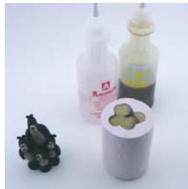
3. The open time of most Alumilite resins is 90 seconds. The color change is the end of the open time and the point in which it will turn color and begin setting up. The finished color of Alumilite Regular is an opaque tan (white and black resin is available along with coloring dyes to color the resin yourself).
