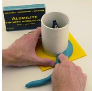
3. Make a mold box out of plastic, wood, metal, poster board, PVC, or any other cup or container. Leave .25"-.375" between your mold box and your original. Seal your mold box with Alumilite's Synthetic Modeling Clay to prevent the mixed silicone rubber from leaking out of your mold box before it cures.
