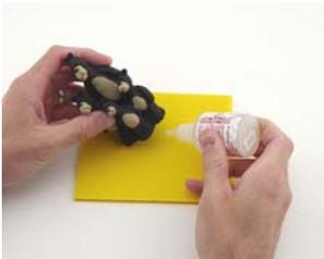
2. Fasten the flat side of your original to a piece of plastic or wood using glue, clay, double sided tape, or super glue. This will prevent the original from floating after you pour the silicone mold making rubber over it. The flat side will give you a nice open area to pour in.
