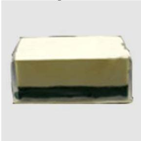
All of the Dow Corning silicone that we carry is mixed 10 parts base to 1 part catalyst (measured by weight). Be certain to completely mix your silicone. Any portion that isn't mixed will not cure. The rubber will be fully cured in 24 hours (only 4-8 hours if you use the Alumilite Quickset RTV).
