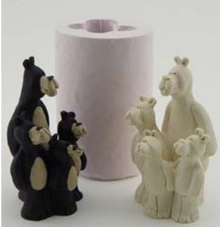
4. Once the resin has hardened (approx. 5 minutes), flex the mold and remove your perfectly cast piece. Your piece is now ready to be painted, sanded, or tapped.
