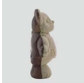
Try to put this in the place where it will be noticed the least. We have decided to have the part go down the side of the bear to avoid seeing it from the front (picture on the right shaded where the front and back halves of the mold will meet). We will pour the part from the least cosmetic place on the original, which would be the bottom of the bear's feet.
