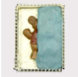
Once you have completely removed the clay, coat the rubber with Alumilite's Rubber to Rubber Mold Release. This will prevent the second layer of silicone rubber from adhering to the first. Vaseline works great for this if you do not have any of rubber-to-rubber release. **DO NOT MOLD RELEASE THE ORIGINAL** and be sure not to miss any rubber sections of your mold. Any area not coated with release agent will stick and will require cutting to separate the two halves apart.
