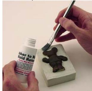
Note: Silicone Rubber will not stick to anything (including your original) other than another silicone rubber. To have the second half of the mold release from the first, you must have a mold release in between the layers where ever the two halves will touch. Including the outside portions of the mold next to the mold box.
