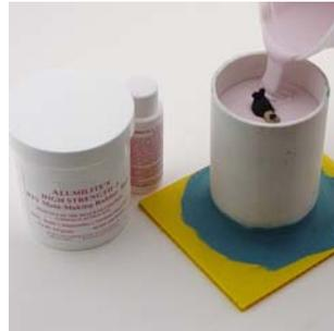
4. Measure the silicone rubber according to the instructions provided with the silicone and mix thoroughly. Once mixed thoroughly, slowly pour the rubber from one corner of your mold box allowing the silicone to flow naturally around your piece. (We have chosen to use HS III due to the large undercuts - bear's chins)
