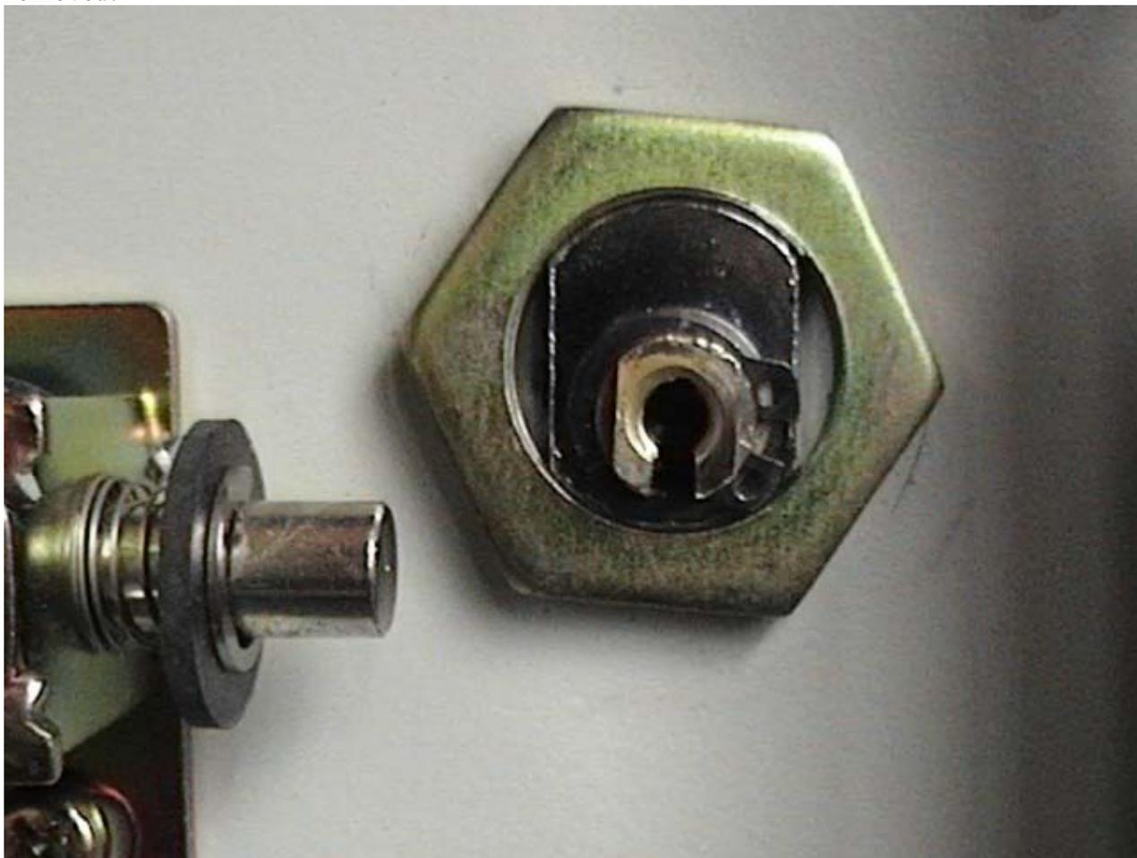
**Step Four- remove the large nut holding the lock in the door; the red arrow points to the nut.**
