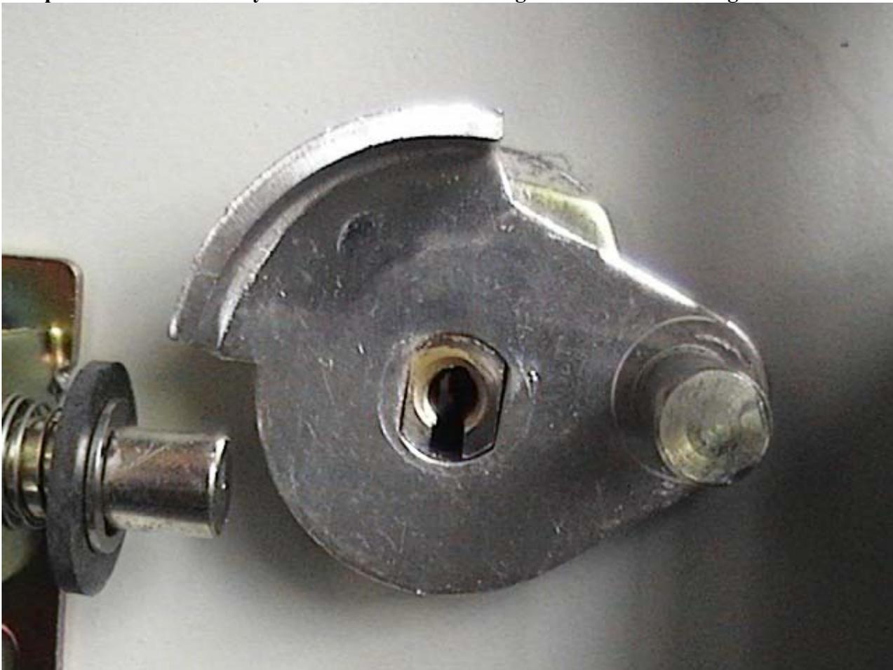
**Step Three- remove the lock tailpiece in the above picture. The picture below shows the tailpiece removed.**
