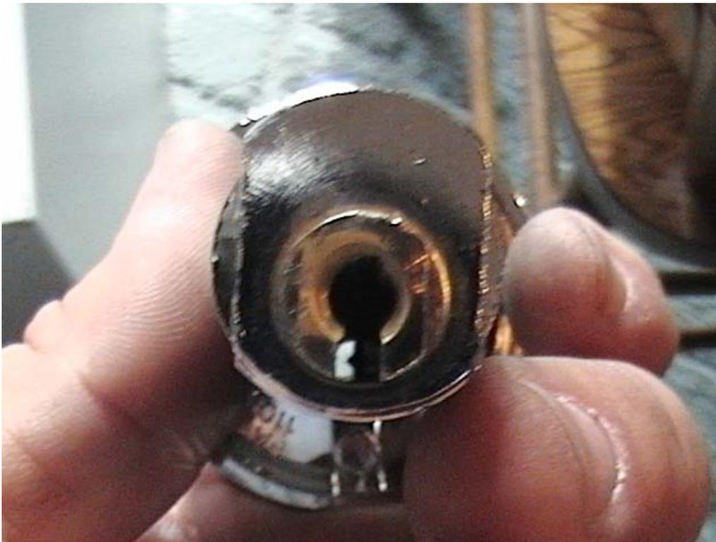
**Step two- remove the plug, you need to pick the pins at the same time and walk the plug out of the front of the shell. I didn't have a follower at the time so I improvised with .375 highlighter pen casing, it needs to be about 4 inches long.**
