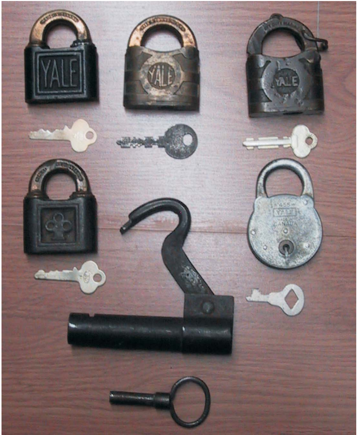
Padlock (?) At bottom the key has Female Tread Turning Clockwise will lock Padlock
