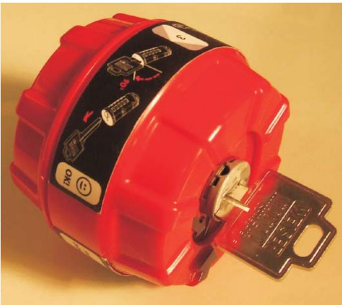
Insert the key you want to use in the cylinder, while making sure not to rotate the cylinder.
