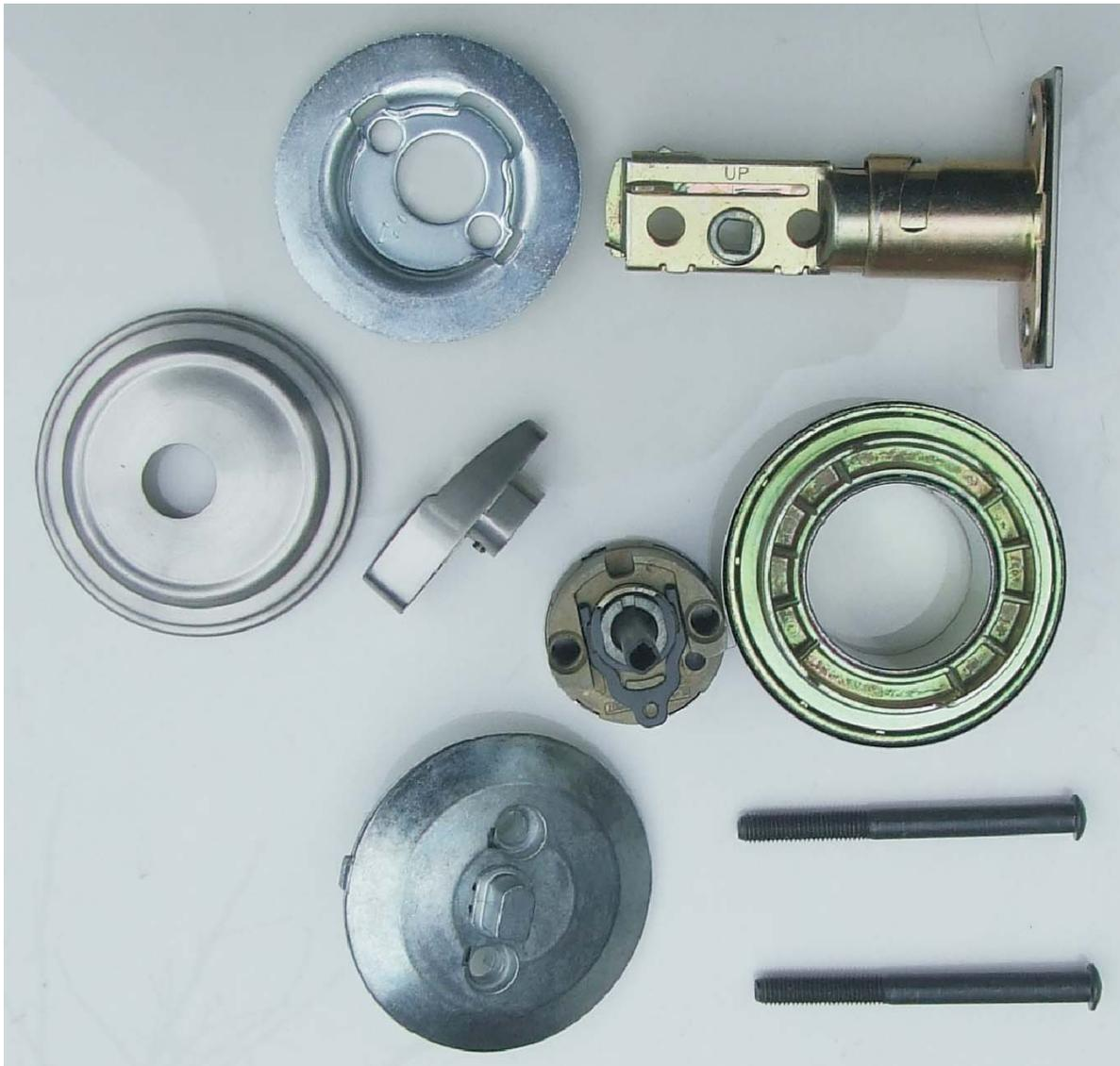
Exploded view of the New SmartKey Weiser deadbolt: the bolt (adjustable), "E" clip and tailpiece are the same as those used on Kwikset. The factory Weiser key has a square head like regular Weiser, although slightly larger.
