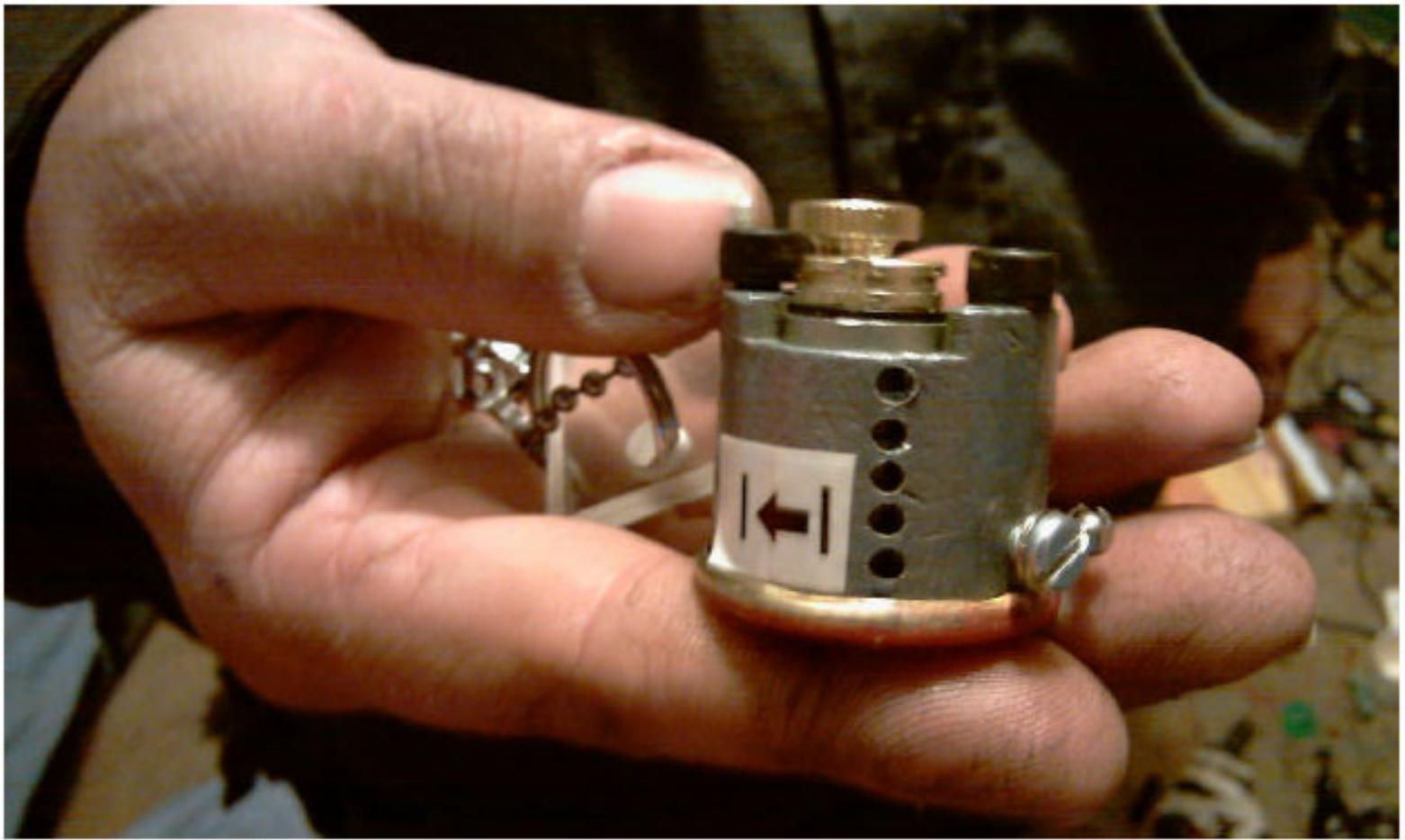
**To use this reset cradle device, insert the cylinder and secure it with the knurled brass nut, holding in the correct position for resetting.**
