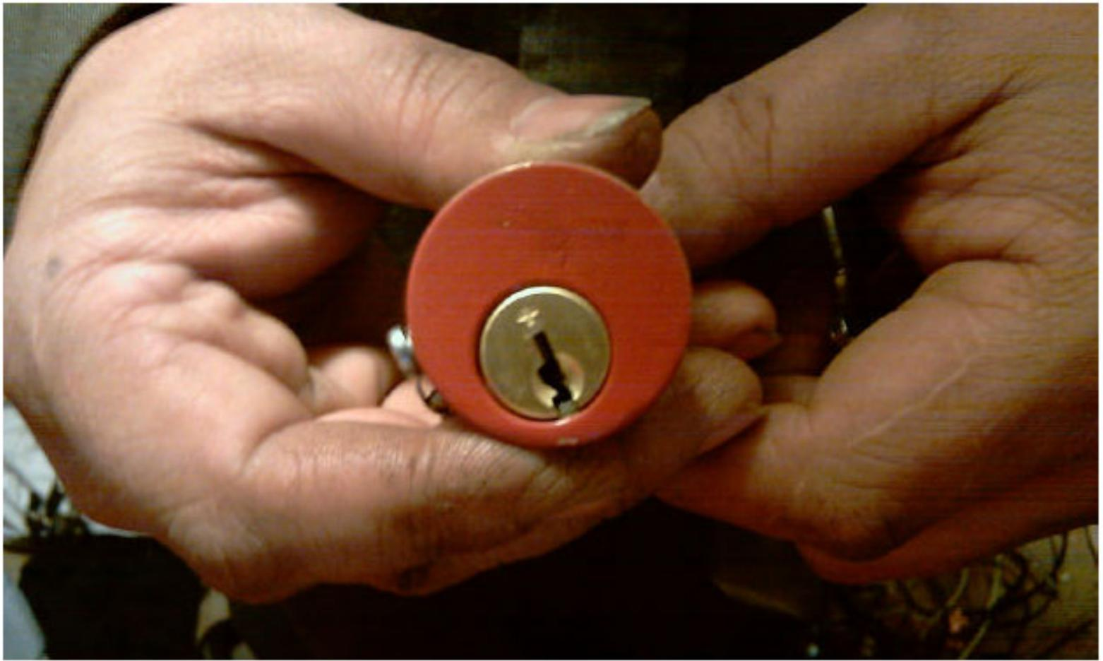
**After resetting to the desired operating key, unscrew the knurled brass nut, and remove the Securekey cylinder from the reset cradle device.**
