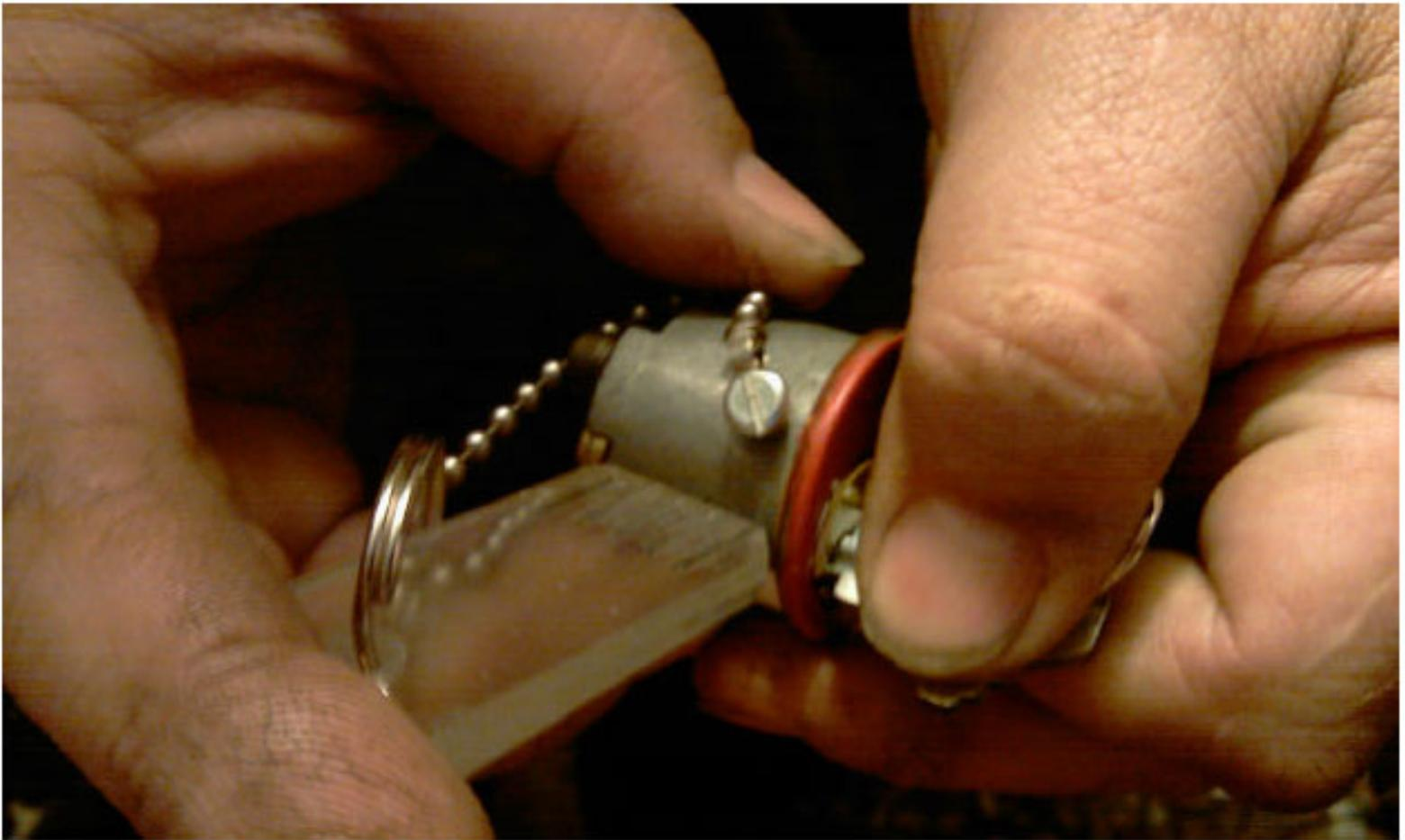
**Once the key and plug begin turning, the comb can be removed, and the plug and key can be turned to the 11 o'clock position, the cut-down blue key is removed, and the cylinder is readied to be reset to the desired operating key using a properly cut blue reset key.**
