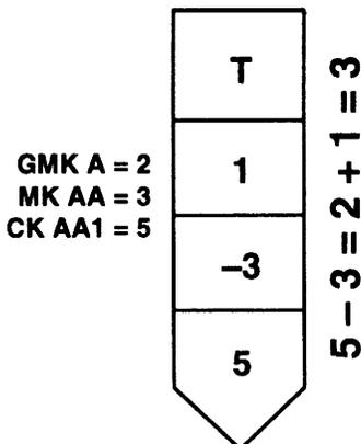
**Example 2:** When the shallowest master key is *deeper* than the change key, the difference is positive, so a +2 build-up pin is required. Both master keys are the same depth in this example, so no master pin is used.
