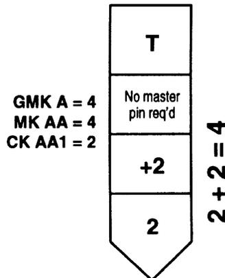
**Example 3:** When the shallowest MK cut is the same as the change key cut, a "zero" build-up pin results.
