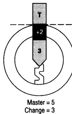
In the second example the change key is still a #3 cut but we've made the master key deeper: #5.
