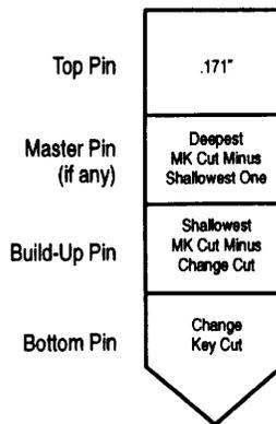
To determine the build-up pin, subtract the change key cut (bottom pin) from the shallowest master cut. The master pin size is the difference (if any) between the deep and shallow master key cuts. The top pin size is a uniform .171" in master ring cylinders.
