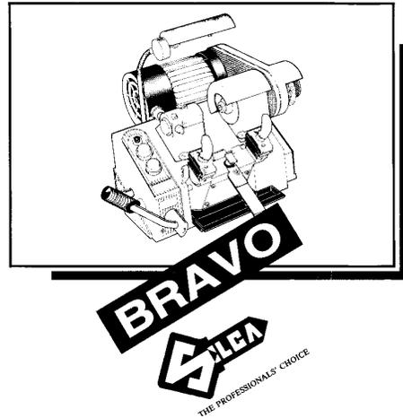
Professional key cutting machine for cutting car and house hold cylinder keys and crucifix keys.
